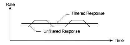
As a guideline to the degree of filtering to be used, the following table shows the response to a step change in input. The value, A, is the filter constant which is set during the configuration process. The times for the display value to reach 90% and 99% of full swing are given in seconds for different values of A.
